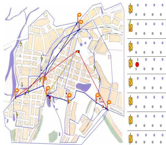
Fig.3. the simulation of electric-taxi DAR operation scheme.
